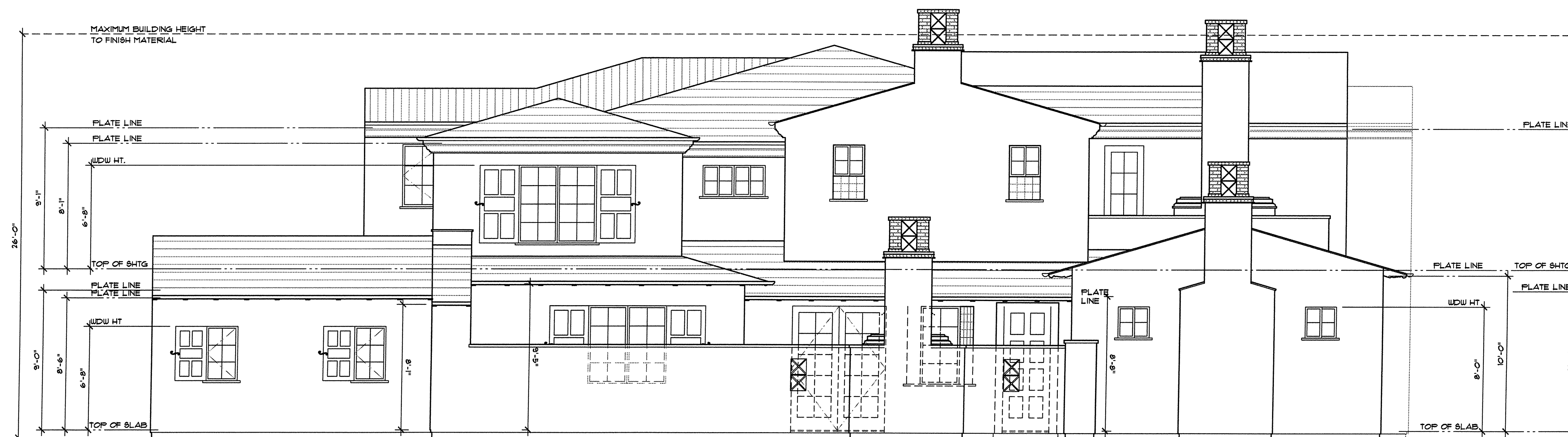
FOURPLEX RIGHT SIDE ELEVATION SCALE: 1/4"=1'-0"
